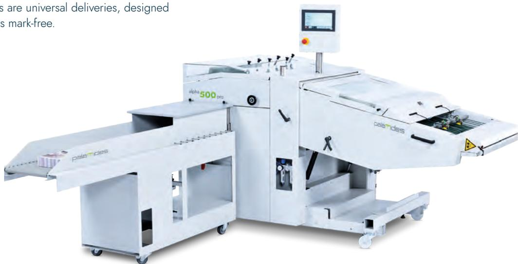
The alpha is a mobile stacking delivery system for mark-free deliveries. It was developed as a universal delivery system for processing folded brochures, specifically signatures and is the standard delivery system on the market for signature processing. It can be coupled with almost all folding machines.
